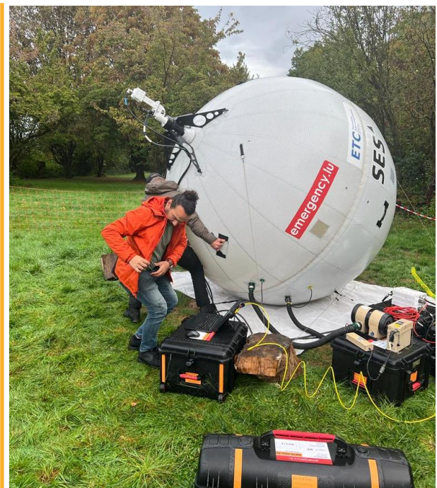
ETC and global partners set up VSAT data connectivity for communication services for responders in Taldad following the earthquake. Photo: Mufaro Masuka
