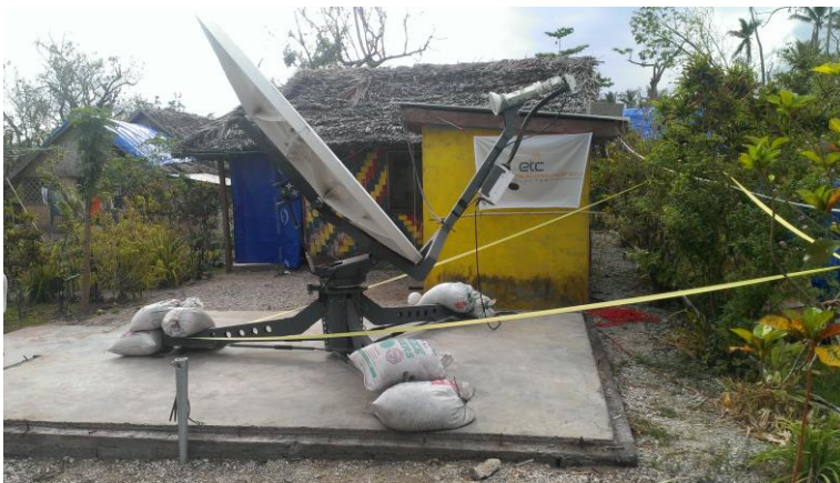
emergency.lu VSAT and Ericsson Response WIDER equipment on Tanna (Tafea Province) is providing connectivity to over 140 humanitarian users. Photo: Ericsson response/ Michael Duffin
